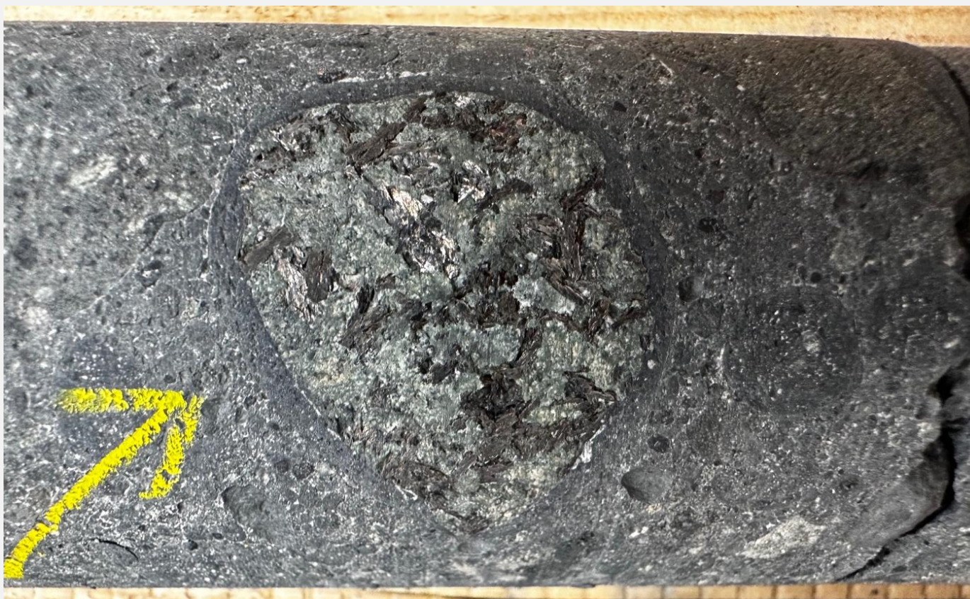
KPK rock at 317 m in drill hole NW23-003, with olivine-phlogopite peridotite xenolith with a thin accretionary magma crust. It is surrounded by unsorted, fine to coarse magmaclasts, spherules and xenolith fragments in a kimberlitic pyroclastic breccia groundmass.
