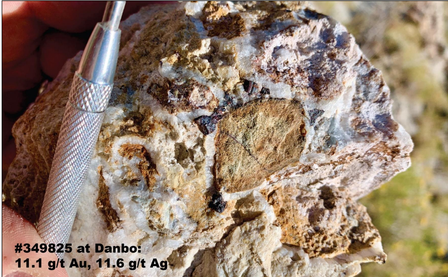
Danbo Property Sulfide-bearing epithermal quartz vein with drusy open space (33.9 g/t Au).
